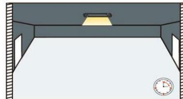
③ After elapse of hold time, the sensor dims the light at the present low light
