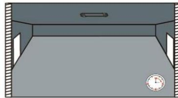
③ After elapse of hold time, the sensor switches off the light when no motion is detected
